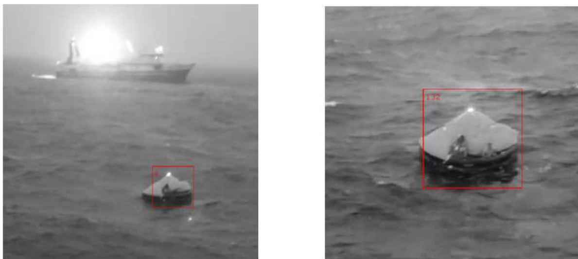
Fig. 5. Evaluation of the trained life raft detector on the real data (rescue operation of the Russian-flagged fishing trawler Dalniy Vostok in 2015)
