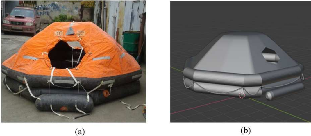
Fig. 3. The life raft PSN-10: (a) the source image of the raft, (b) the 3D model of PSN-10
