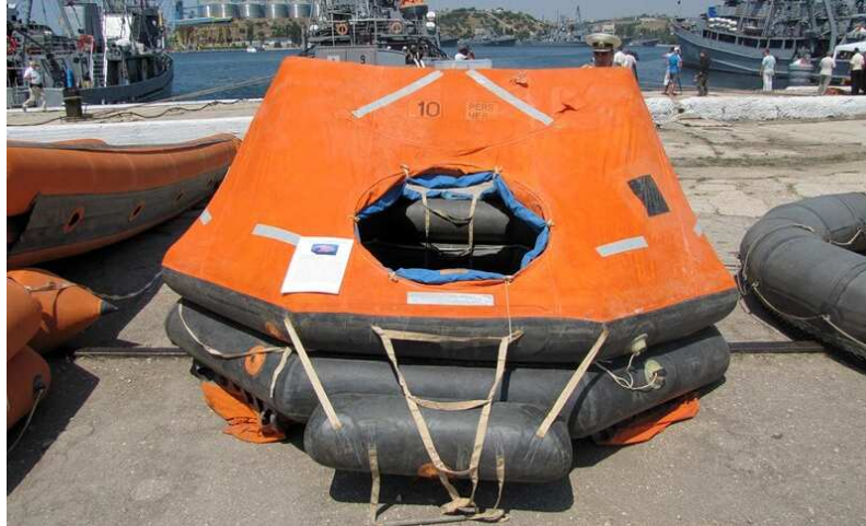
Fig. 1. A sample of the inflatable life raft PSN-10
